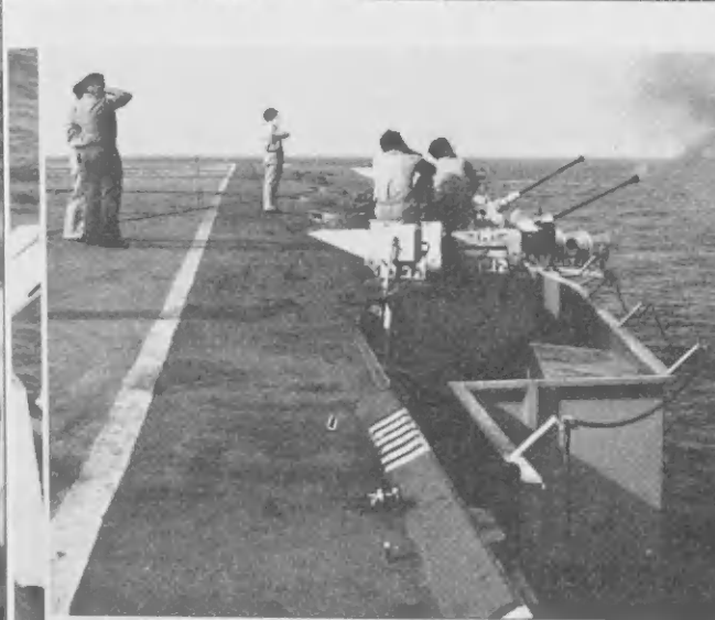
THE ARMAMENT of the HRMS Karel Doorman includes ten 40mm anti-aircraft guns. The guns are positioned in wells which extend beyond the flight deck. E ARMAMENTO di HRMS Karel Doorman ta inclui diez cayon anti-aereo di 40 mm. E cayonnan ta posiciona den poosnan cu ta extende tras di e dek di vuelo di portaavion den awanan.
